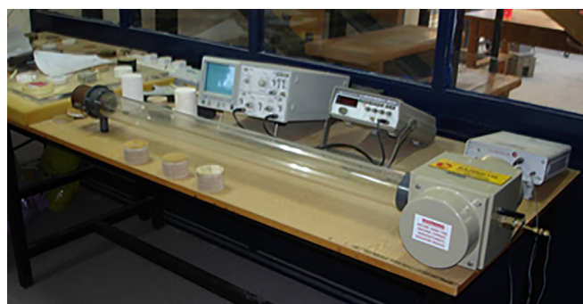
FIG. 5. (Color online) Standing wave tube used in BS 575 course.
