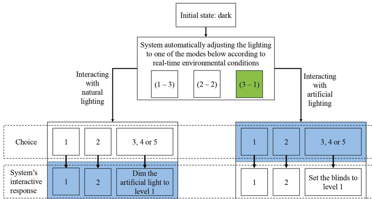
**Fig. 2.** The operation logic diagram of the interactive lighting system in scenario III. The green box represents the automatic lighting setup in the experiment. (For interpretation of the references to color in this figure legend, the reader is referred to the Web version of this article.)
