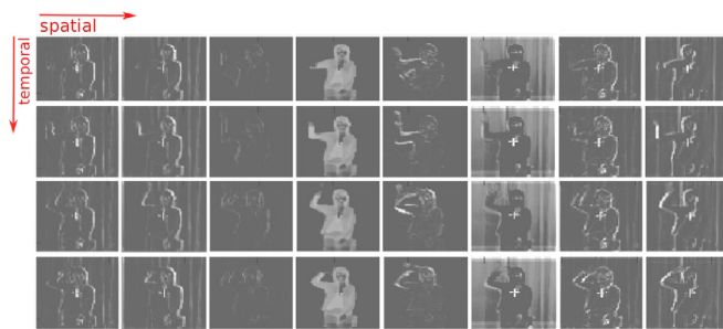
Fig. 4. 3D convolutional neural network model to represent video stimuli. (a) Structure of the 3D Convolutional Neural Network (C3D) model including convolutional, max-pooling, and fully connected layers, and (b) Sample activations from pool1, pool2 and pool3 intermediate layers on handwave video stimulus.
