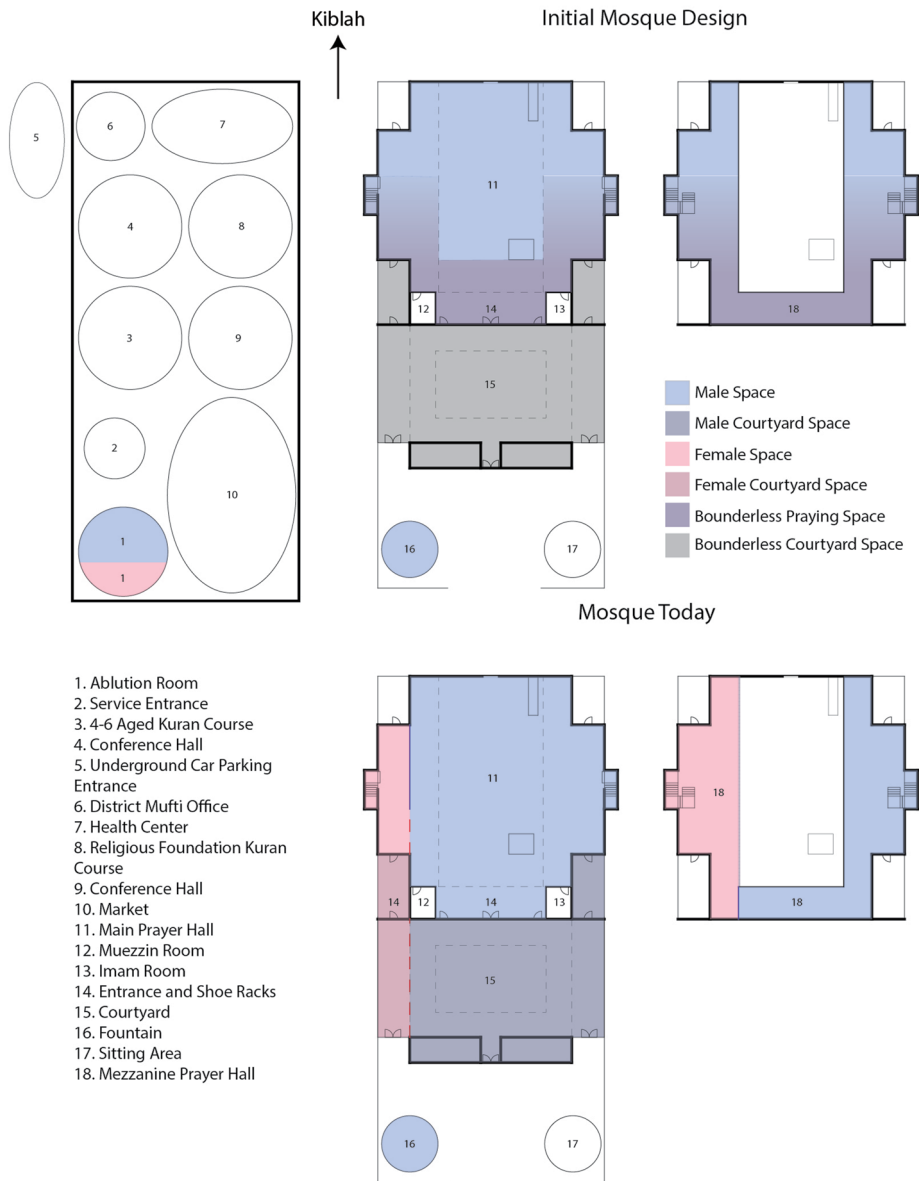
Figure 5. The functions and space usage based on gender in the Çamlıca Mosque.
