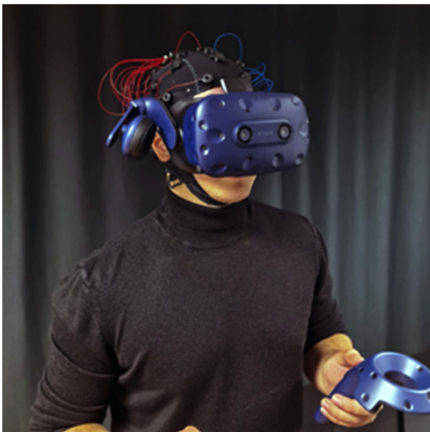
Figure 6 Participants Were Wearing the EEG Headset and the VR HTC Vive Pro
