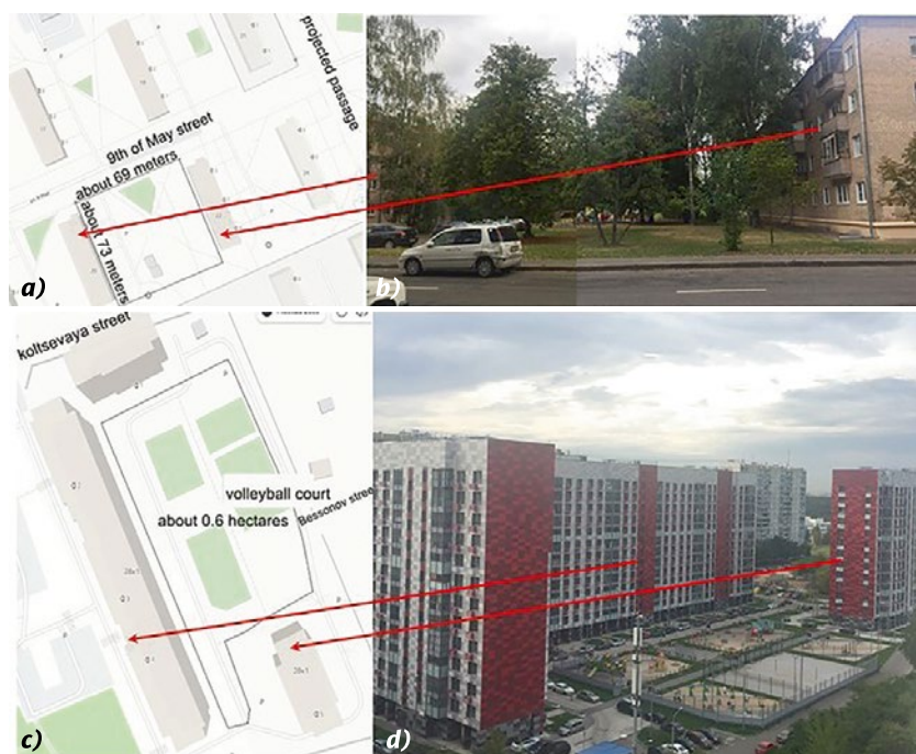
Fig. 3. Impact of the building density of the territory on the architectural appearance of the living environment, Eastern settlement, Moscow: a) line building with inter-house territory of about 0.4 ha; (building density (2.8–3.2) thousands m 2 /ha) with 4-storey residential buildings, year 1962; b) general view of the territory with an abundance of greenery and sufficient space for quiet and active recreation; the first launch pad for demolition under the renovation program; c) compensation development for renovation (with density about (17–20) thousands m 2 /ha); d) functional and planning organization of the residential complex territory on Main Street (year 2022) on the site of the former green zone as part of the renovation program (photos and drawings by L.A. Solodilova)
